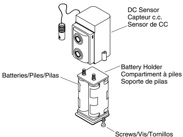
**NOTE:** Replace the batteries when the LED continuously flashes when a user is in sensor range.
