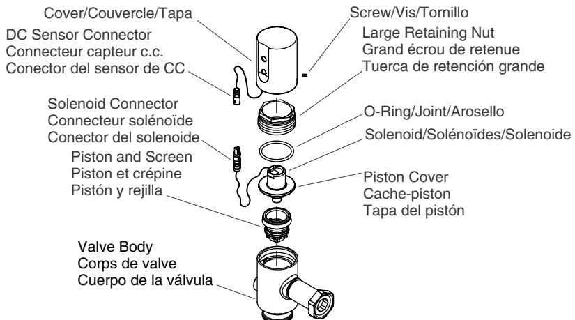
**NOTE:** The screen, located within the piston, is designed to keep debris from clogging the bleed hole. The screen may require periodic cleaning.
