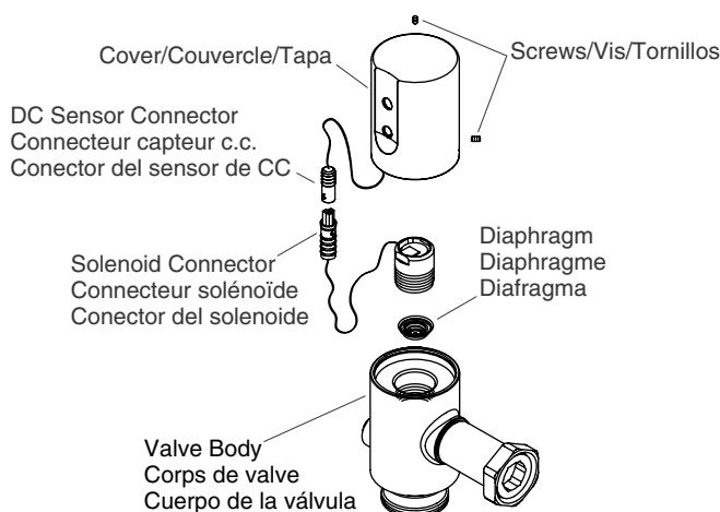
**NOTICE:** To avoid product damage, ensure the wires do not get caught between the cap and the valve body.
